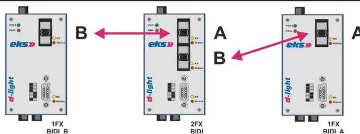
Systems with BIDI transceivers always have to be connected from transceiver type A to a transceiver type B. Switches with 2 FX-Ports always have transceiver type A as the upper one.
